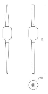
$\begin{array}{c} \text{dimensions}: \textit{Ø}~28~x~h~205~cm \\ \text{LED}~source \end{array}$
